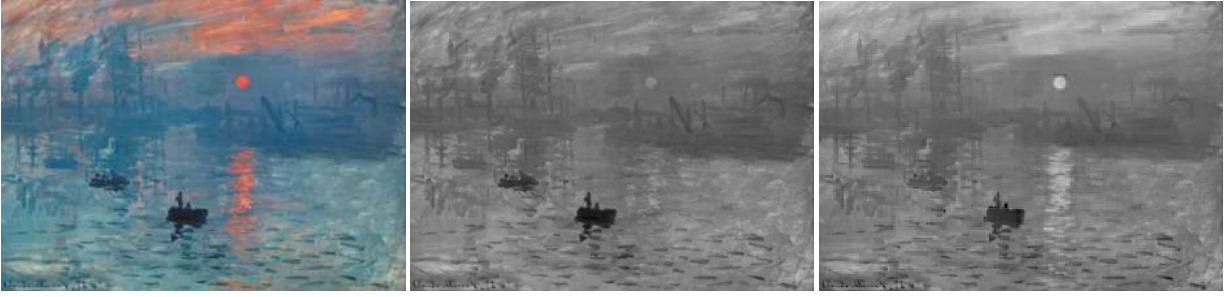
Figure 15: An example of a saliency preserving color to gray mapping. Left – original image; center – luminance image; right – the result of the color to gray algorithm. Image: Impressionist Sunrise by Claude Monet
