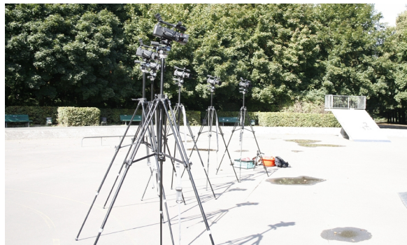
Figure 1: Recording setup: for our STF/X editor, consumer-grade camcorders suffice. The setup is flexible: adjacent cameras are only required to have sufficient view overlap and the angle between viewing directions should not exceed 10 degrees.
