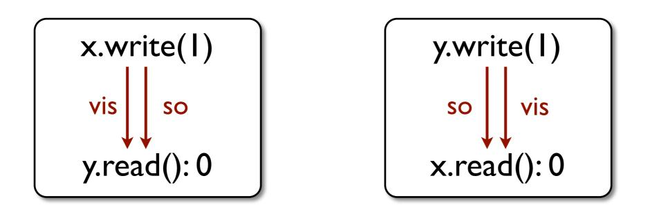
Not serializable, allowed by transactional causal consistency and parallel snapshot isolation
