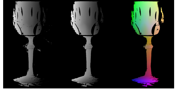
Figure 12: Scan maps generated from space-time stack. From left to right: depth map t(u, v) before and after segment size filtering, world coordinate map (x, y, z) . Colors are normalized for print.
