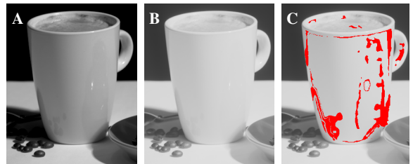
Figure 5: Detail Visibility. HDR image (A) contains subtle reflection on a surface of the cup. A global tone mapping (B) reveals the coffee beans in the shadow but the reflection details become indiscernible. The areas of image with lost details are predicted by our metric (C), where red colour marks \Delta T^* > 1 .
