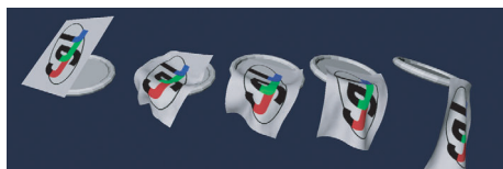
Figure 2: The two-side collision detection allows to work with open meshes. Here the cloth falls and then slides onto a plate.
