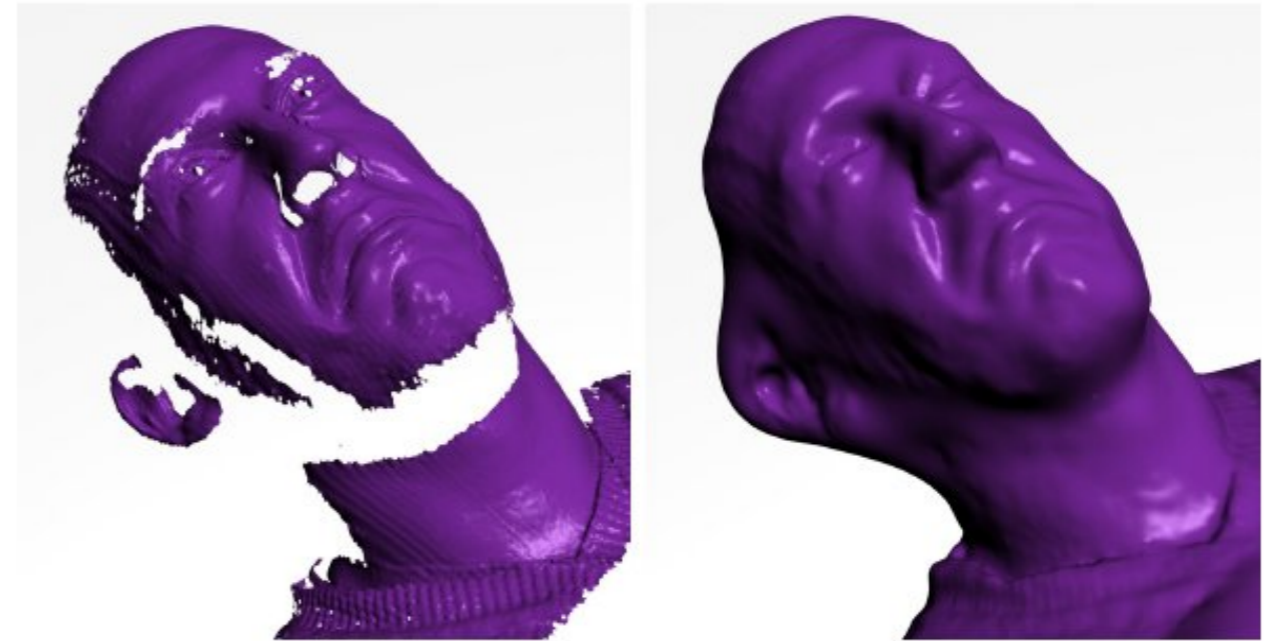
Figure 4: Holes due to occlusions in the scanning process (left) are filled by the implicit surface (right).
