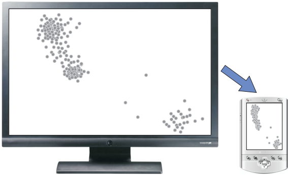
Fig. 1. A distribution of a conventional scatterplot to both a large and a small display (or a scatterplot has been re-distributed from a large to a small display) often causes trouble with visual effectiveness: users may perceive a different number of clusters
