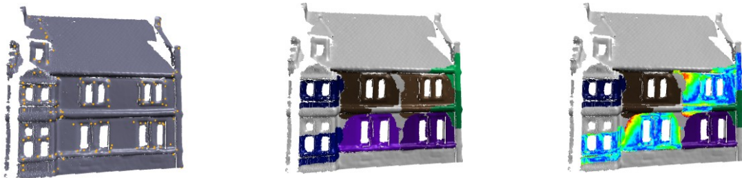
(d) Clay house model: Left detected features, middle: symmetric parts (instances are color coded), right: matching residuals.
