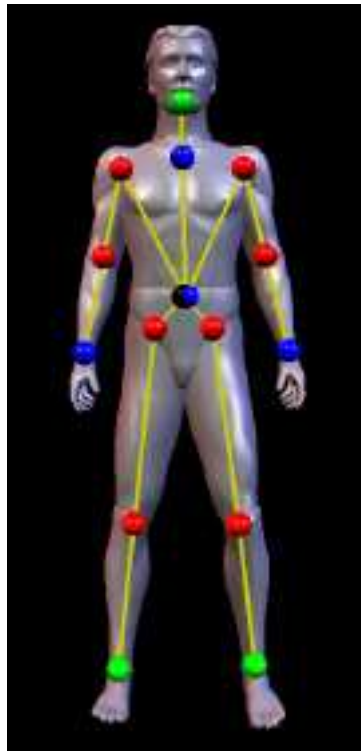
Figure 3.2: The surface model with underlying skeleton. Spheres indicate joints and the different parameterization for each. Green sphere - 1DOF, blue sphere - 3 DOF, and red sphere - 4DOF. The blue-black sphere at the pelvis represents 3 joints simultaneously, one for the root and the other two to connect the upper and lower parts of the model.
