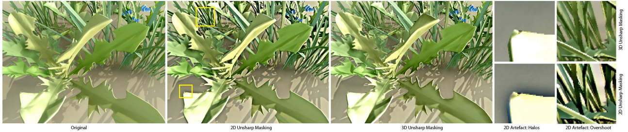
Figure 1. Traditional vs. 3D Unsharp Masking. From left to right: Original Image; Enhanced version by traditional unsharp masking ( \lambda = 1.0, \sigma = 8.0 ); Enhanced version by 3D Unsharp Masking. Note that traditional Unsharp Masking overdoes the enhancement in some regions breaking scene-coherence (right). The 3D version preserves scene-coherence.
