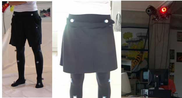
Fig. 12.18. The set-up for quantitative error analysis: Left/middle, the subject with attached markers. The cloth does not interfere with tracking the markers. Right: A strobe light camera of the used Motion Analysis system.
