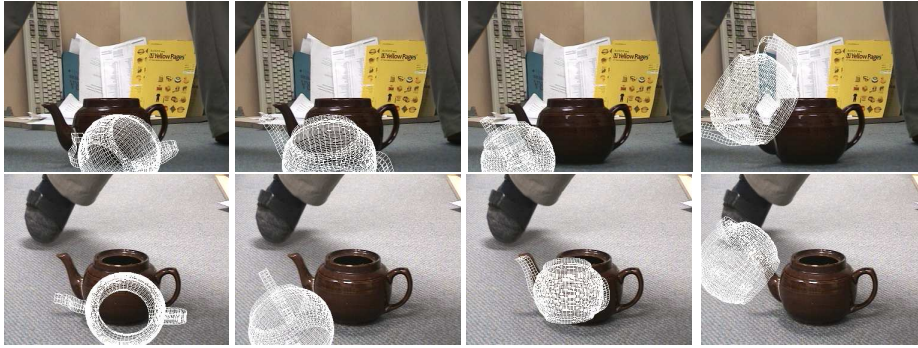
Fig. 6. Example rotations, which still converged using the ICP+OF algorithm but failed with ICP alone.
