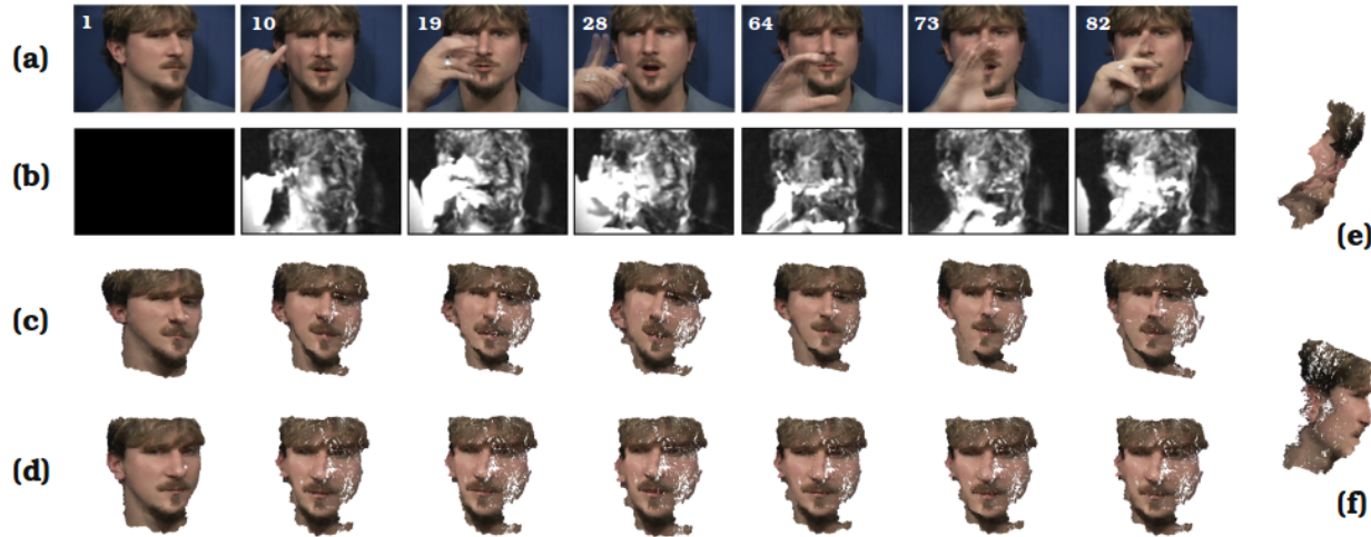
Figure 4: Experimental results for the ASL sequence [1]: (a) reference frame 1 and several frames with occlusions; (b) corresponding occlusion maps; (c) reconstructions with MFSF[3]+VA[2]; (d) reconstructions with MFSF[3]+SPVA (per frame per pixel); (e) side view of frame 28 for the configuration used in (c); (f) side view of frame 28 for the configuration used in (d).
