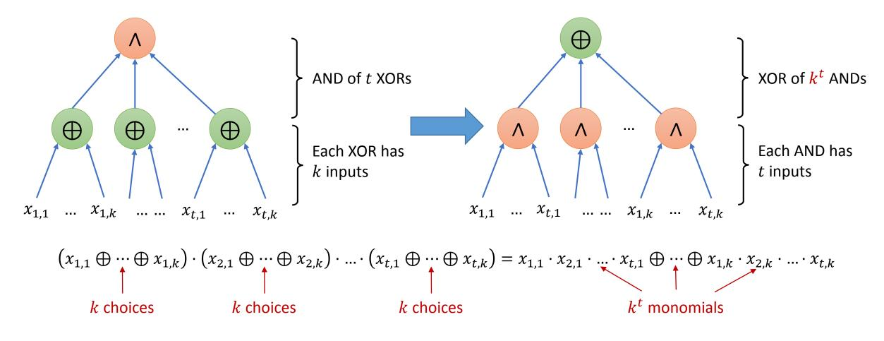
Running time:  $O(k^t t \cdot deg)$  where deg is degree after expansion (maximum size of any monomial); here deg  $\leq t$
