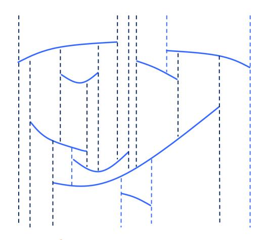
trapezoidation G to obtain <u>smaller</u> G' remove set of independent segments and "retrapezoidalize" holes repeat recursively
