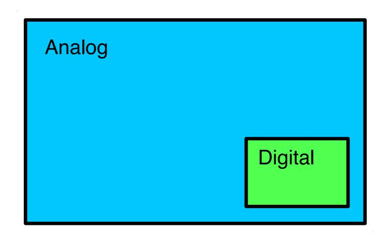
Digital filter can be 10x smaller than analog filter: large capacitances required by analog filter.
